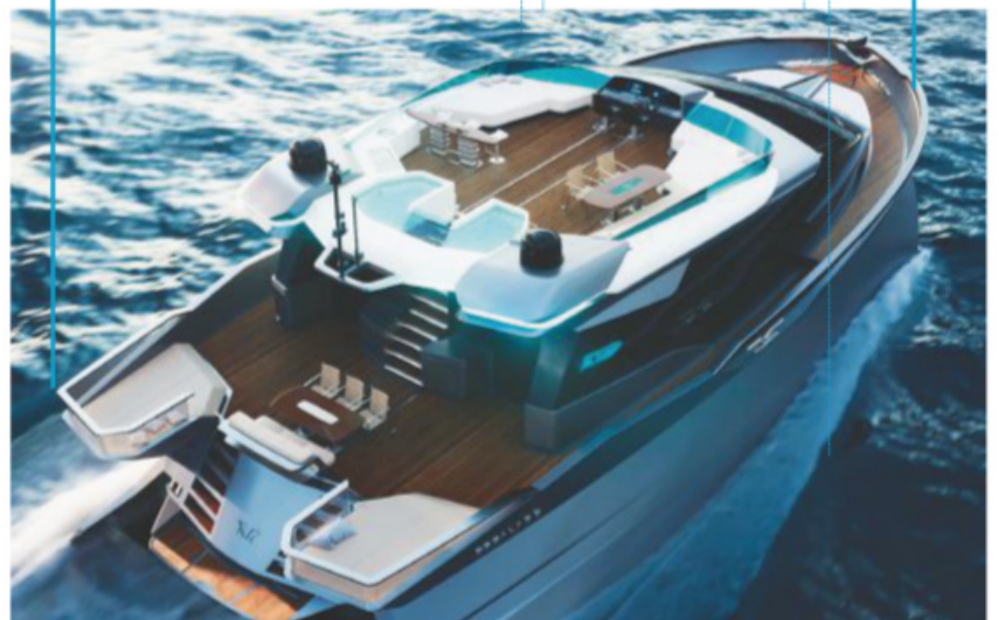
LEFT Project Escalade features a radical new trimonoran hull INSET Designer Baran Akalin penned its futuristic lines ABOVE AND BELOW The three hulls are linked by foils at the bow and stern
